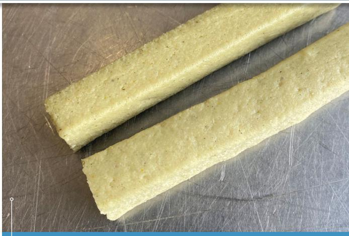
This dental stick is produced by utilizing a single-screw extruder, a mid-barrel valve, and our advanced densification unit (ADU) to achieve optimal texture and durability.
