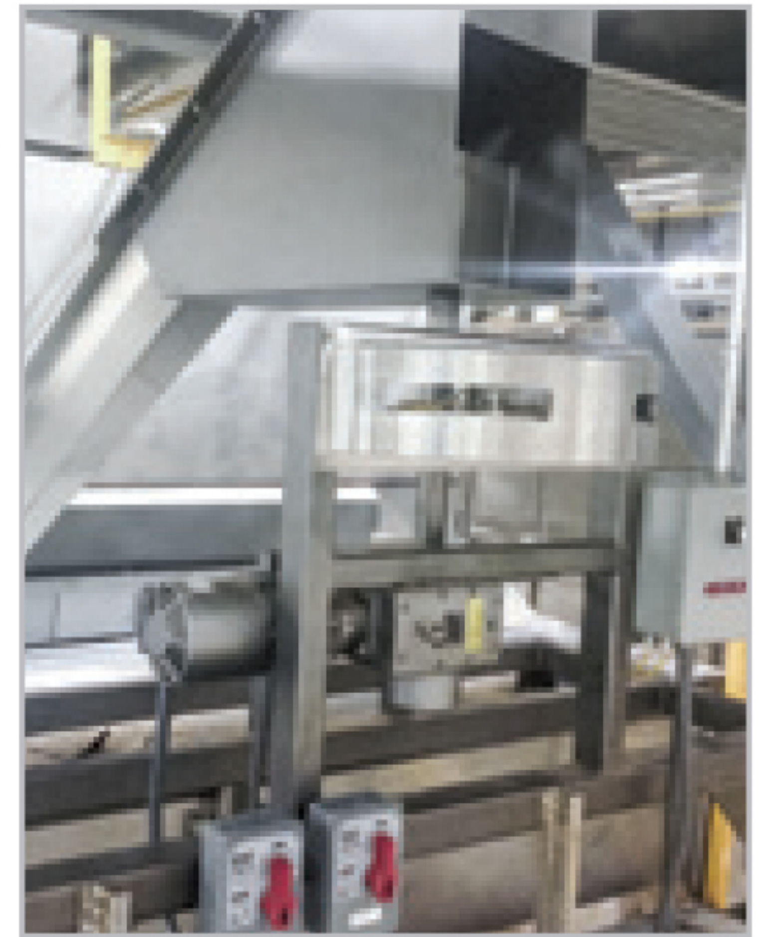
Redesigned chute with span and speed controls for "in-process" adjustments, reduced horizontal ledges allow for ease of cleaning
