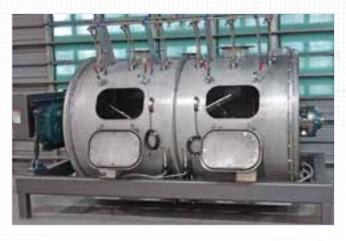
Coatings are applied in our enclosed batch mixer that features best in class product coating coverage and optimized throughput all with reduced potential for cross contamination.
