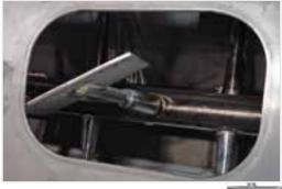
Unique rotary paddle design allows gentle material handling and reduces product degradation.
