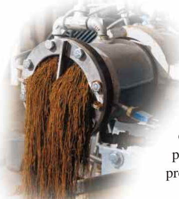
Agglomerated strands are produced utilizing a low shear, low heat extrusion process.
